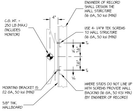
Tu = 152 LB/SCREW (MAX) Vu = 135 LB/SCREW (MAX) SIDE ELEVATION AT STEEL STUD WALL
