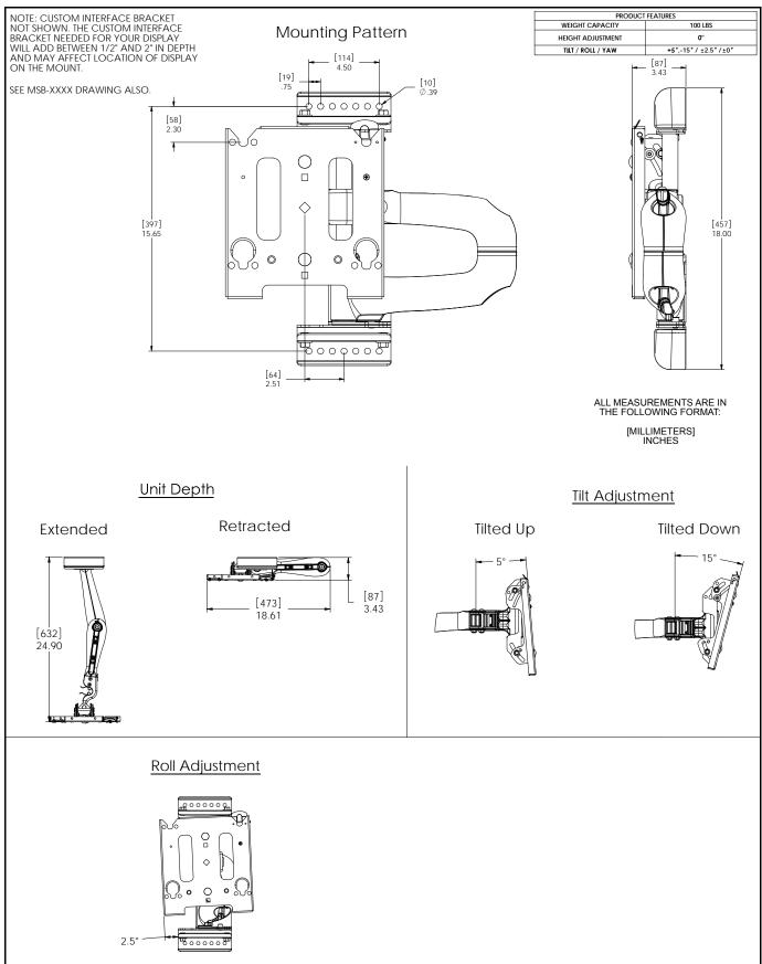
WARNING: IMPROPER INSTALLATION CAN LEAD TO MOUNT FALLING CAUSING SERIOUS PERSONAL INJURY OR DAMAGE TO EQUIPMENT! It is the installer's responsibility to make sure the structure to which the MWH is being installed is capable of supporting five times the combined weight of the mount and all attachments.
