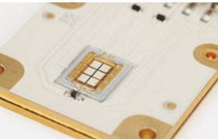
◀ Redundant LED design offers fail-safe operation.
